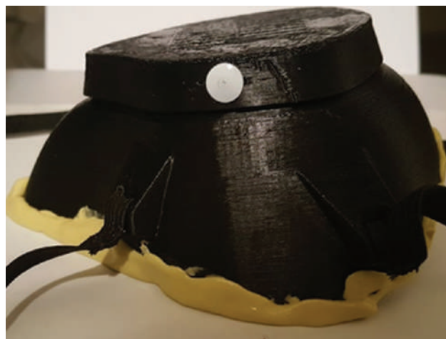
Fig. 9. Additional fixing of the cover using office tacks and addition of a heavy silicone flexible seal to the Lowells Makes mask printed in PLA
